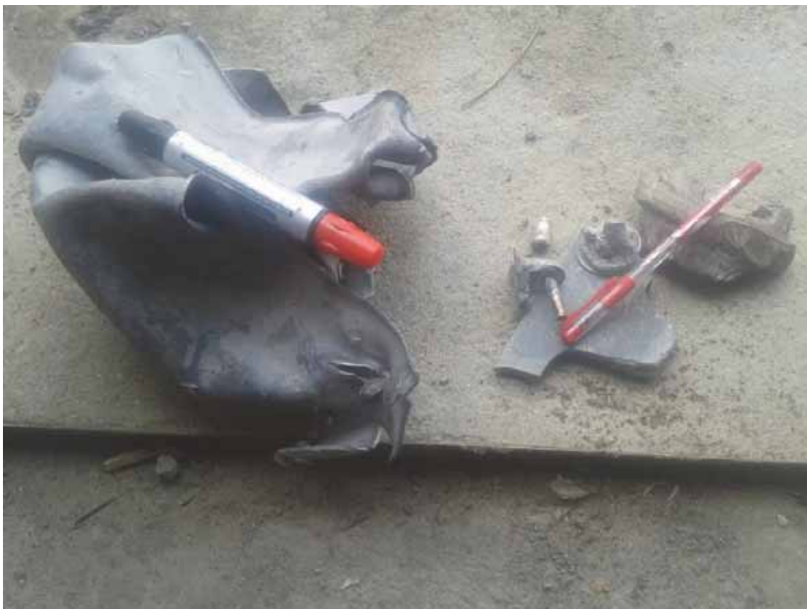
Remnants of a US-made Joint Direct Attack Munition (JDAM) satellite guidance kit, which is fitted to an airdropped bomb prior to use, identified at the site of a wedding bombed by coalition aircraft in Hajjah governorate on April 22, 2018. The strike killed 22 people, including eight children, and wounded at least 54 others, including 26 children. © 2018 Abdo Show'ai
